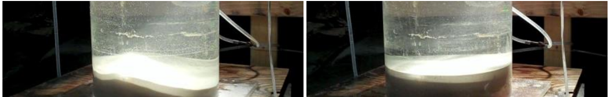
Figure 9: The sediment bed after conducting a high flow rate Washout Performance test on a 90 degree outlet sump. (Left) Without a SAFL Baffle and (Right) with a SAFL Baffle installed at 90 degrees with respect to the inlet pipe (From McIntire et al. 2012).
