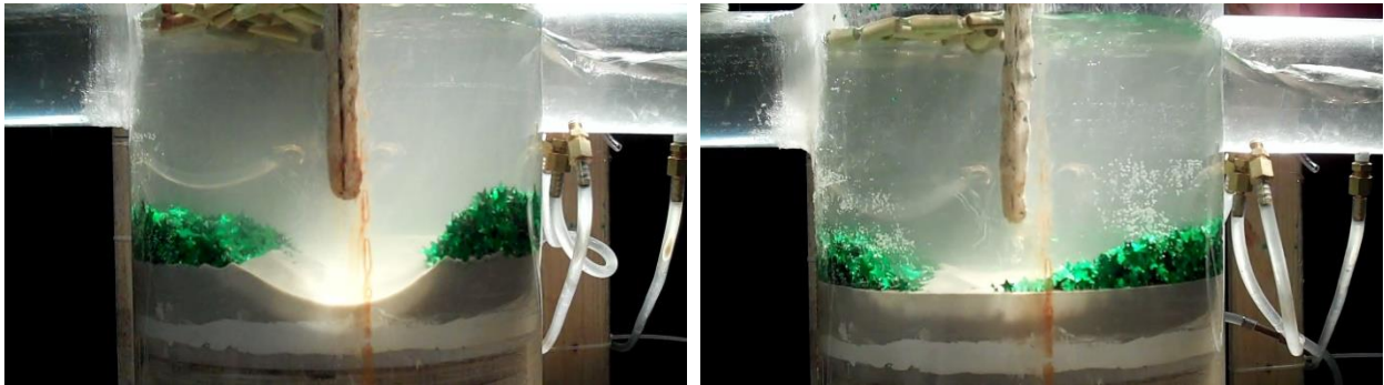
Figure 5: Washout of sediment measured due to debris clogging the SAFL Baffle. (Left) A 3 inch hole diameter SAFL Baffle installed in a sump manhole and (Right) a 5 inch hole diameter SAFL Baffle installed in a sump manhole (From McIntire et al. 2012).
