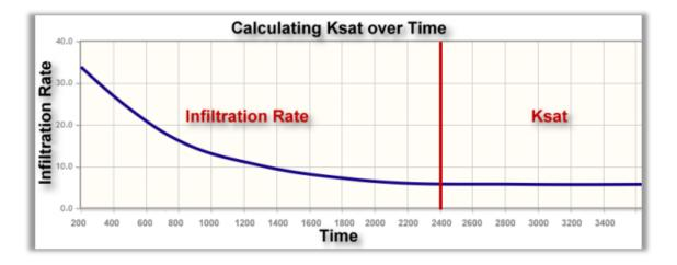
Using the exponentially decaying curve we plotted earlier, we can take just 20% of the data on the far left and apply the Green-Ampt theory to predict Ksat on the far right. This saves time, water, and eliminates any subjectivity as to when 100% saturation has been achieved.
