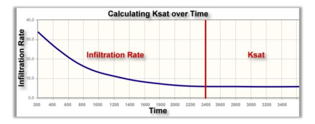
No mater what device is used, (Double Ring, Percolation, MPD or Turf-Tec) the infiltration rate from each, if plotted over time, would be identical.
