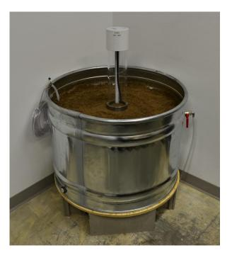
Each MPD test uses approximately 2.5 liters of water. And it takes about 12.5 liters of water to saturate the sand tank to the point where there is standing water above the sand.
