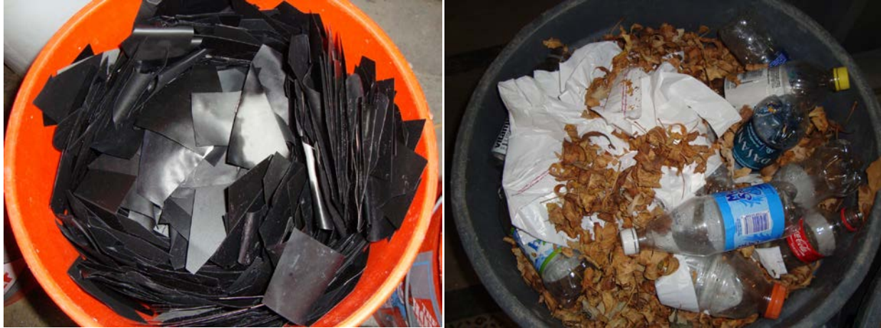
Figure 3-5: Vinyl leaves, plastic grocery bags, and plastic bottles used as simulated debris.
