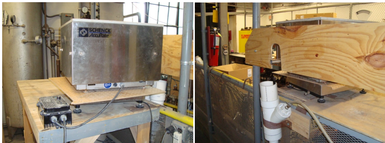
Figure B-1: The Schenck AccuRate feeder loading a slurry of sediment and water into an upstream feed pipe.
