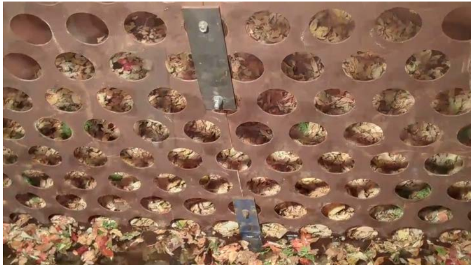
Figure 3-14: Test 2 from the 6×3 washout testing series during its loading phase. The view is from near the outlet pipe, looking upstream.
