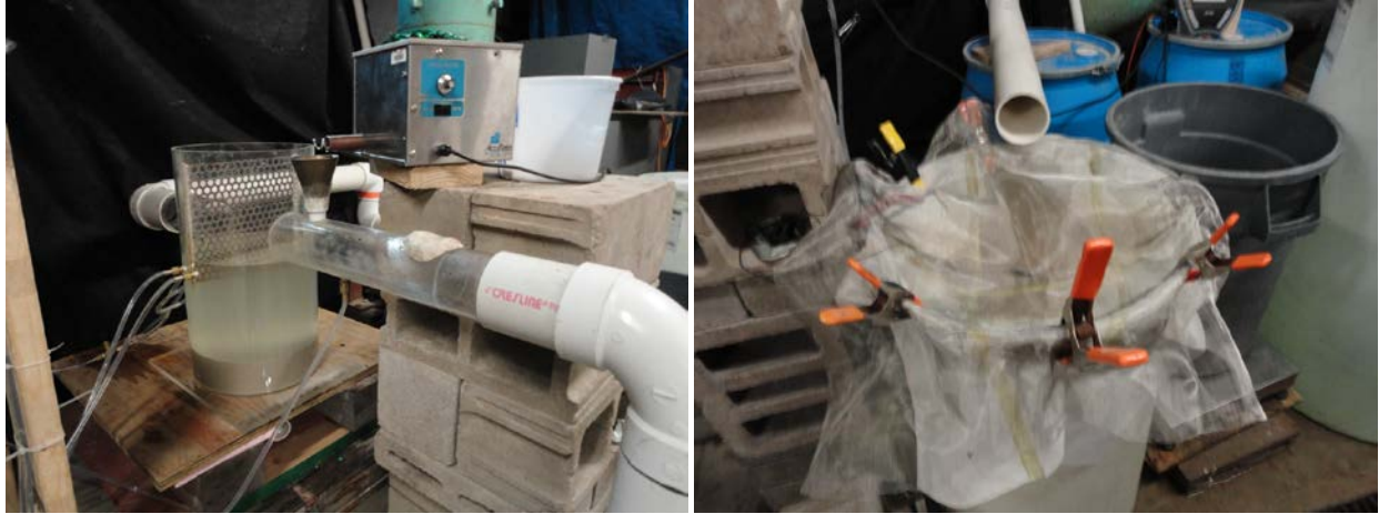
Figure A-6: Scale model testing system. (Left) water travels from right to left through the sump. (Right) water exits the sump through a PVC pipe system and travels into a head tank protected by a mesh screen and 0.00079-in (20 \mu m) filter.
