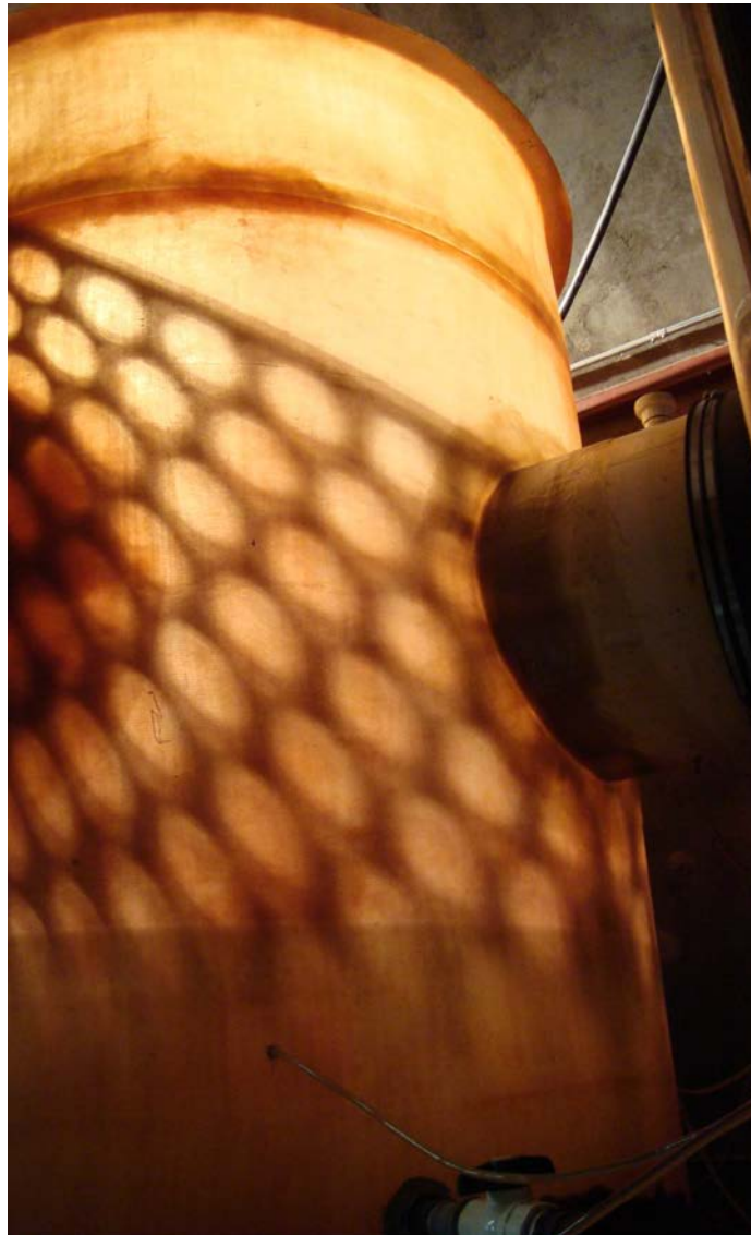
Figure A-3: A view of the 6×6 sump manhole setup. The inlet pipe is to the right and the outlet pipe is not shown in this picture. A shadow of the SAFL Baffle can be seen since the sump is lit from the inside.
