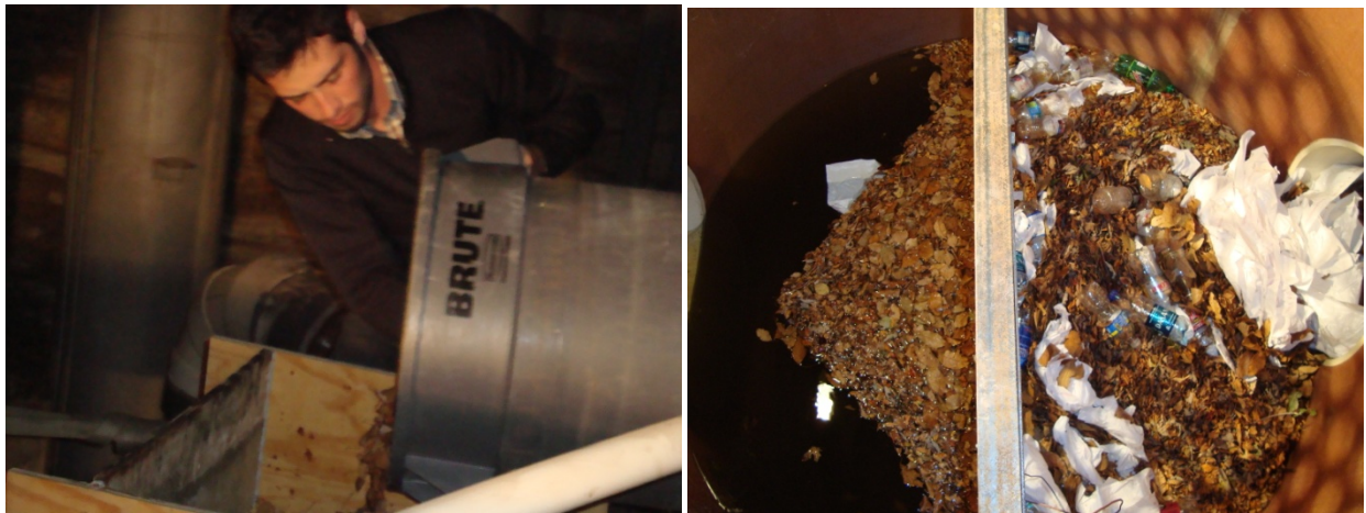
Figure 3-4: (Left) loading simulated debris upstream of the manhole sump. (Right) water leaving the sump's outlet and traveling through the tail box, where debris is collected.
