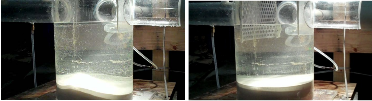
Figure 4-3: Post washout test on the 1×1-90 degree outlet sump without a SAFL Baffle and with a SAFL Baffle oriented at 90 degrees to the inlet pipe.
