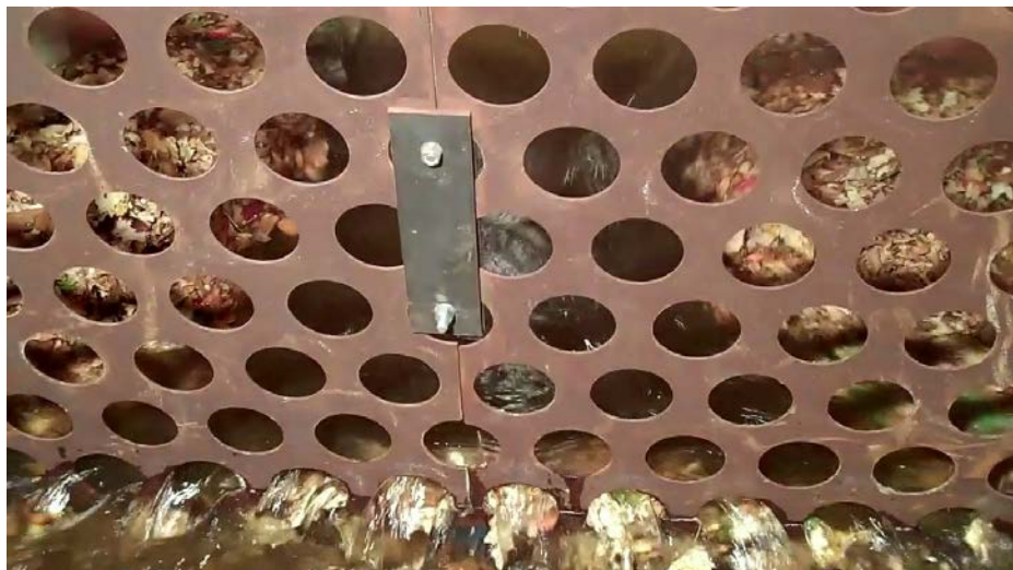
Figure 3-15: Test 2 from the 6×3 washout testing series during its washout phase. The view is from near the outlet pipe, looking upstream.
