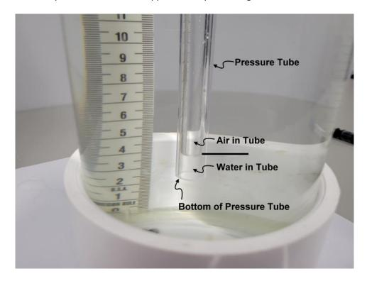
As you place the tube into the water and set the MPD head, the air inside of the tube compresses under pressure, about 0.4 PSI. Approximately 1cm of water will go up inside the tube as shown in the picture above.
